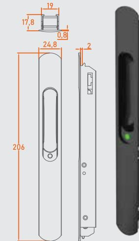
**RECTANGULAR****DESIGNED RECESSED LOCK****DİKDÖRTGEN KESİTLİ****BİLYALI HAVUZ KOL****35.22.004.001**
